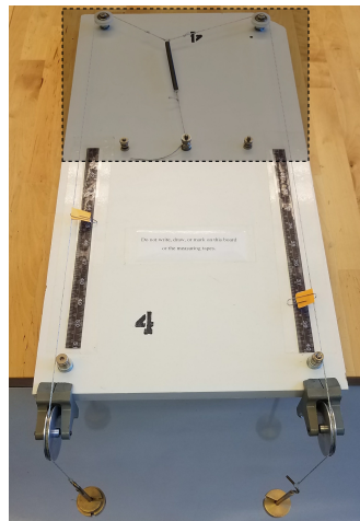
FIG. 1. A Partial Derivative Machine (PDM) with a representation of a black box that can be physically placed on the PDM to hide the system. Two strings emerge from the box/system, each with an associated position (indicated by flag markers) and force (provided by hanging masses).
